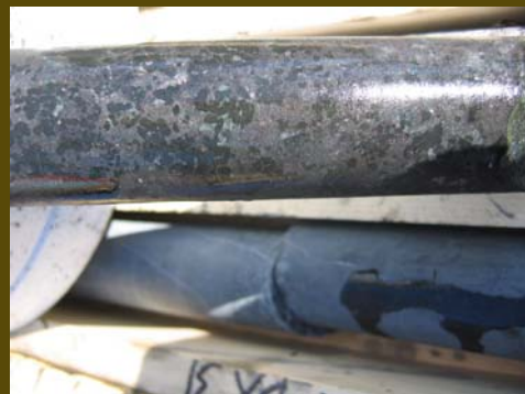
Drill Hole CL-06-12: 19.0 metre intersection grading 0.26% Ni/Cu
