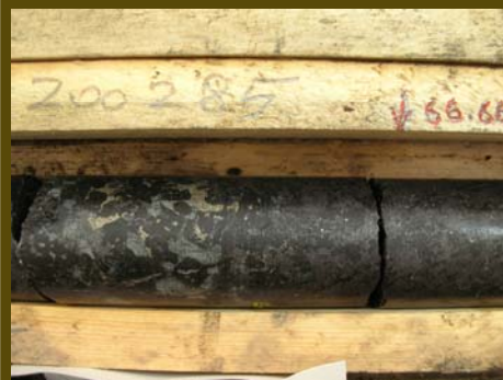
Drill Hole CL-06-39: 69.71 metre intersection grading 0.21% Ni/Cu
