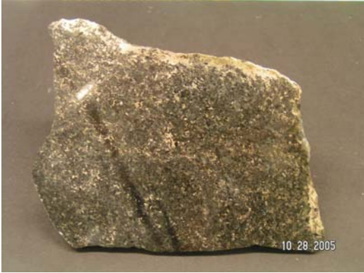
Gabbro with Interstitial and Net-Textured Sulphide, Assayed up to 1% Cu, 0.6% Ni, 0.1% Co
